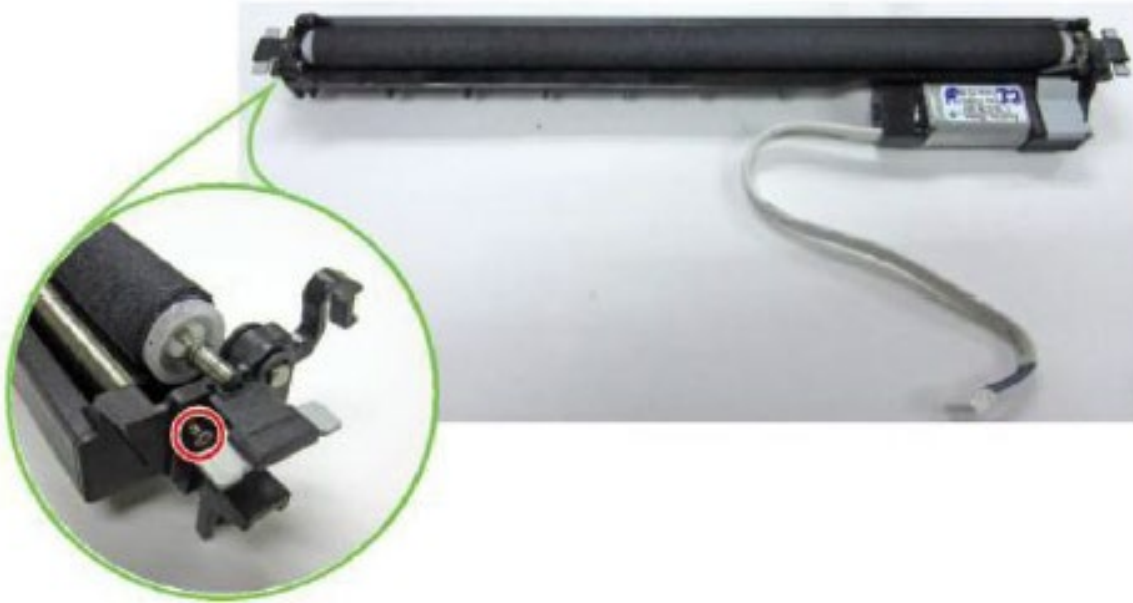
Figure 4, Loosening Screws & Unlocking Latches Holding Micro-Fiber Roller in Place
