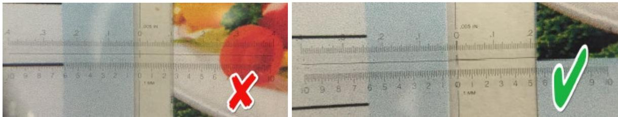
Here is the left label was printed with an increase of 0.06 inches to the length. There is now LESS than 3mm space between the printed data. The right label was also increased 0.06 inches but there is still about 5mm space.
