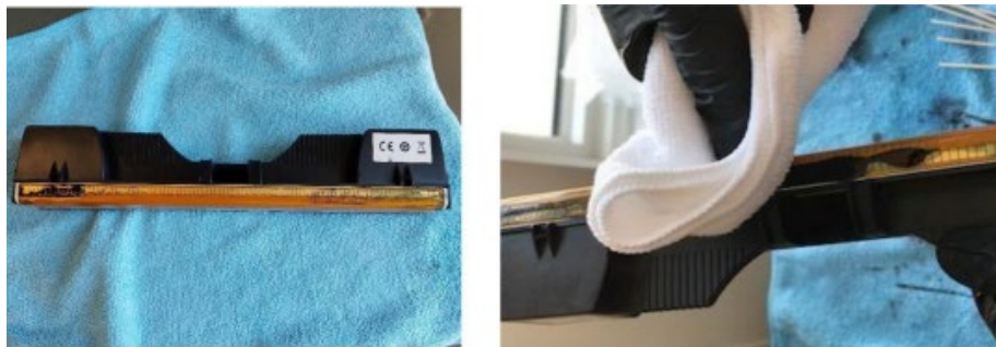
Figure 1. Wiping printhead contacts clear of debris with a dampened microfiber cloth with distilled water.
