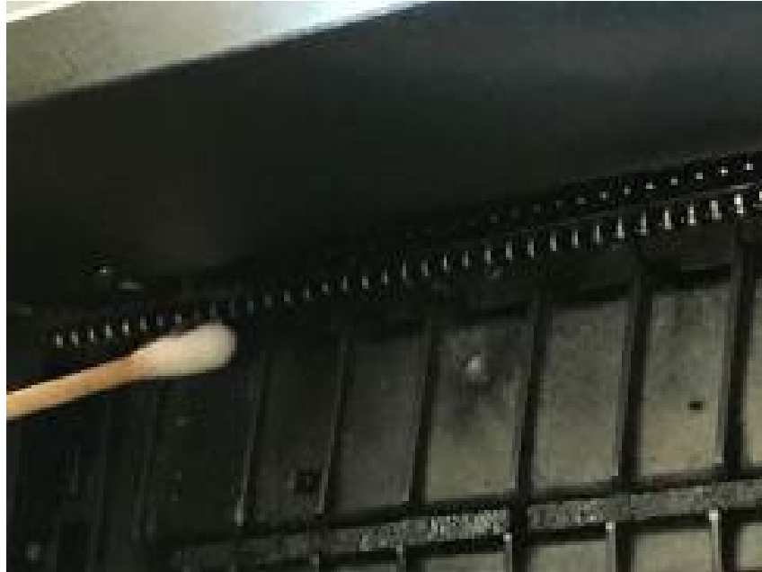
Figure 4. Gently cleaning off Pen PCA board contacts with a cotton swab and a little rubbing alcohol.
