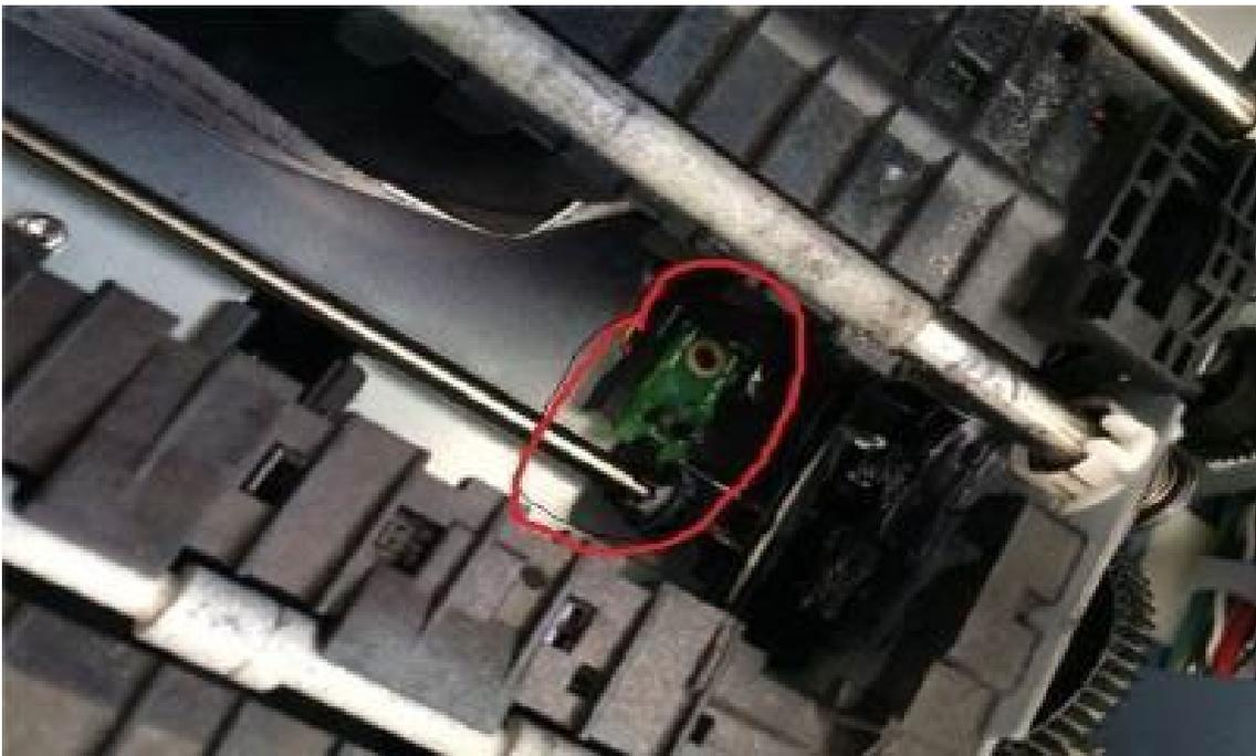
**Figure 1, Identifying and Locating both Goal Post Sensors**
