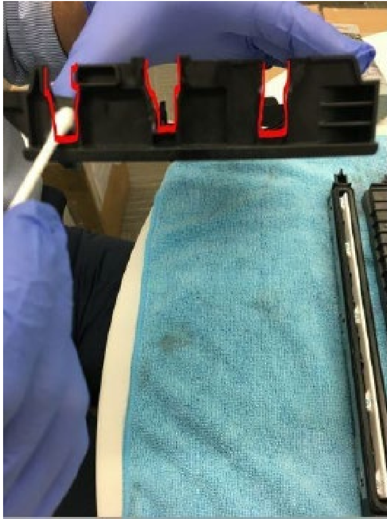
Figure 4, Lubricate the slots marked in red on both sides of the service tray.
