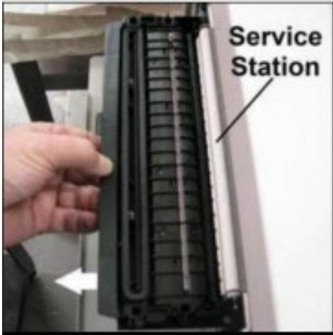
**Figure 1A. Pulling Service Station Out of Printer**
