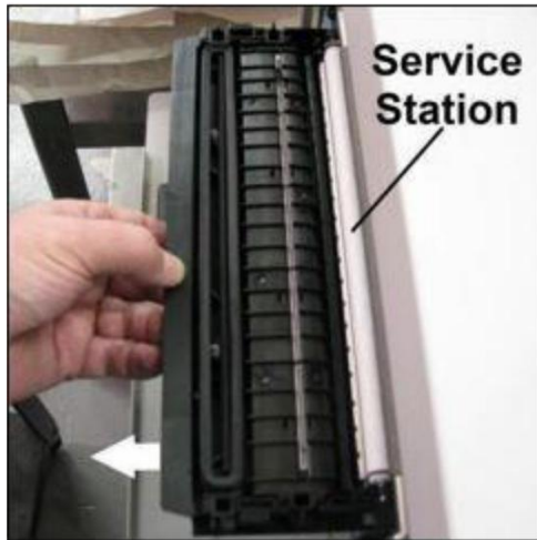
Figure 1A. Pulling service station out of printer
