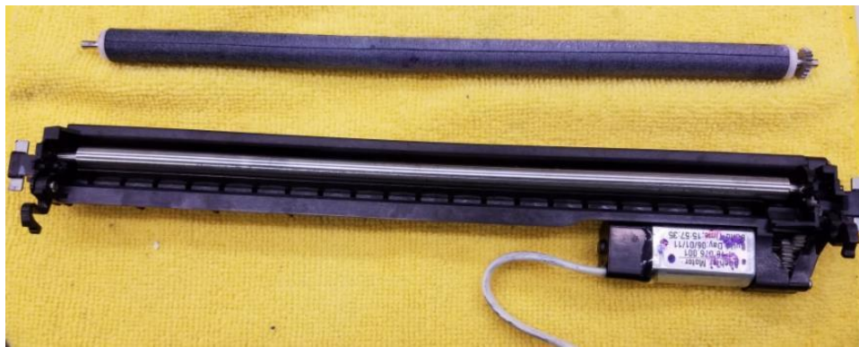
Figure 3. Remove microfiber roller from holster.
