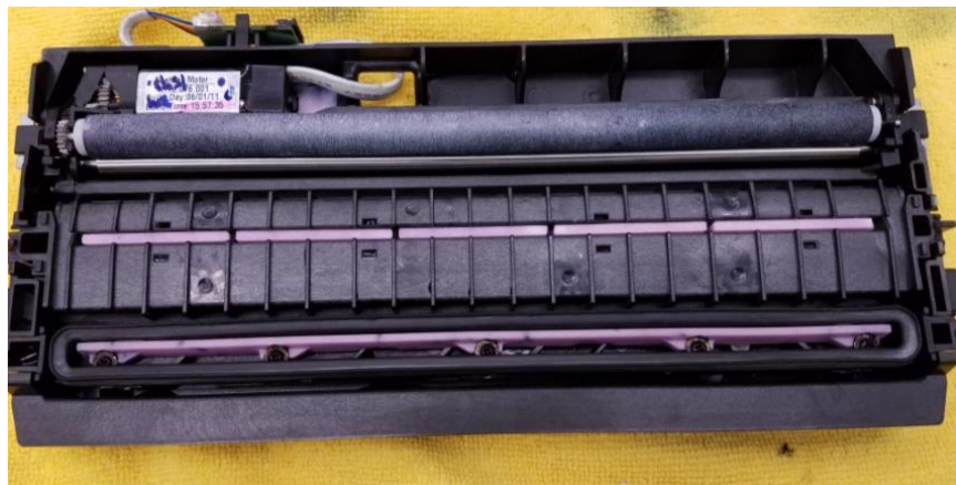
Figure 6. Assembled service tray after being washed
