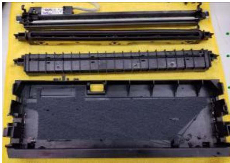
Figure 4. Parts that can be washed in the sink (Platen, Cap & Tray) are marked with green dots.
