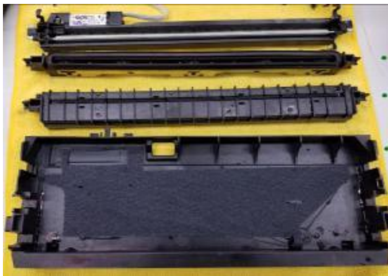
Figure 4. Parts that can be washed in the sink (Platen, Cap & Tray) are marked with green dots. For additional support call the Vivid Data Support Team at 1-855-848-4332 Option 2!
