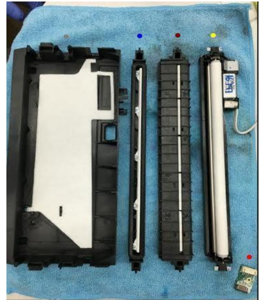
Figure 1. Service Station Components
