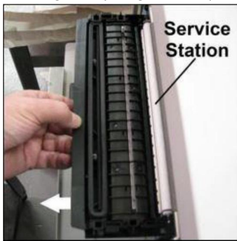
Figure 1. Ejecting service tray
