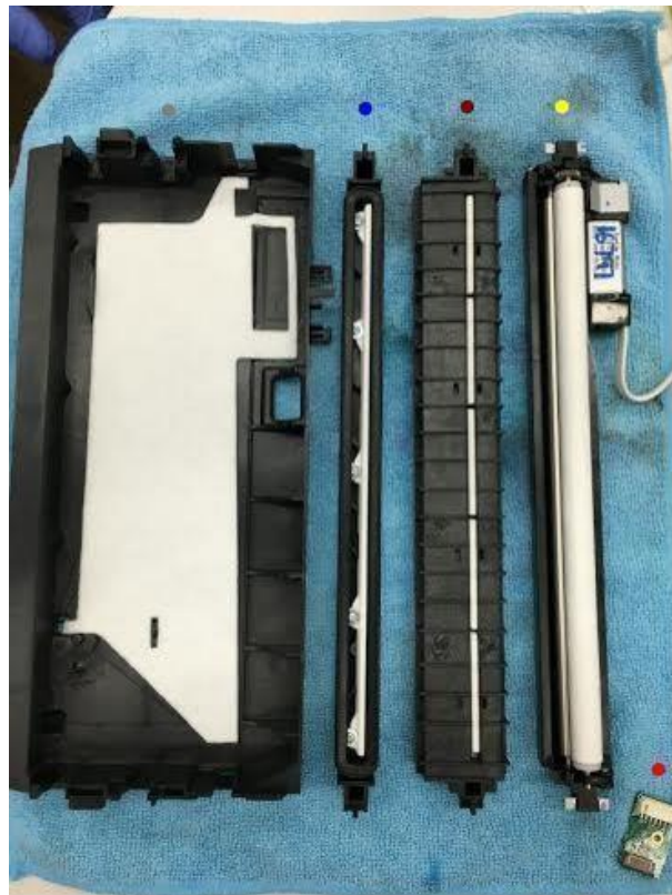
Figure 3. Overview of compartments contained in the service tray
